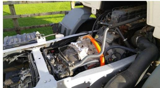
Prototype Commercial Vehicle Motor
